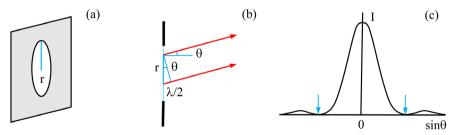
**Figure 5.** (a) Light passing through a small circular opening leads to interference. (b) It is always destructive for a particular angle  $\theta$ . (c) The angular distribution of the resulting light intensity I yields a central blob, surrounded by fainter luminous rings.
