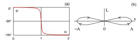
**Figure 12.** (a) The phase difference between the forced oscillation and the applied force. (b) This type of periodic variations of the effective length L of the pendulum yields a parametric amplifier.
