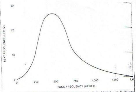
SPECTRUM OF BINAURAL BEATS was measured by J. C. R. Licklider, J. C. Webster and J. M. Hedlum. Rapid heats, up to shout 26 per second, can be heard when the tons used to produce them are about 110 hertz. With tones of higher or lower pitch the manmum heat frequency declines. When the interval exceeds about 30 hertz, two tones are heard
