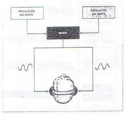
**EXPERIMENTAL METHOD** for generating monaural beats uses two electronic oscillators and a network, her called a mixer, to combine their outputs. Each ear hears a composite signal; the beats can be heard with one ear or both. With the oscillators tuned to the frequencies shown, six beats per second (440 hertz minus 434 hertz) would be perceived.
